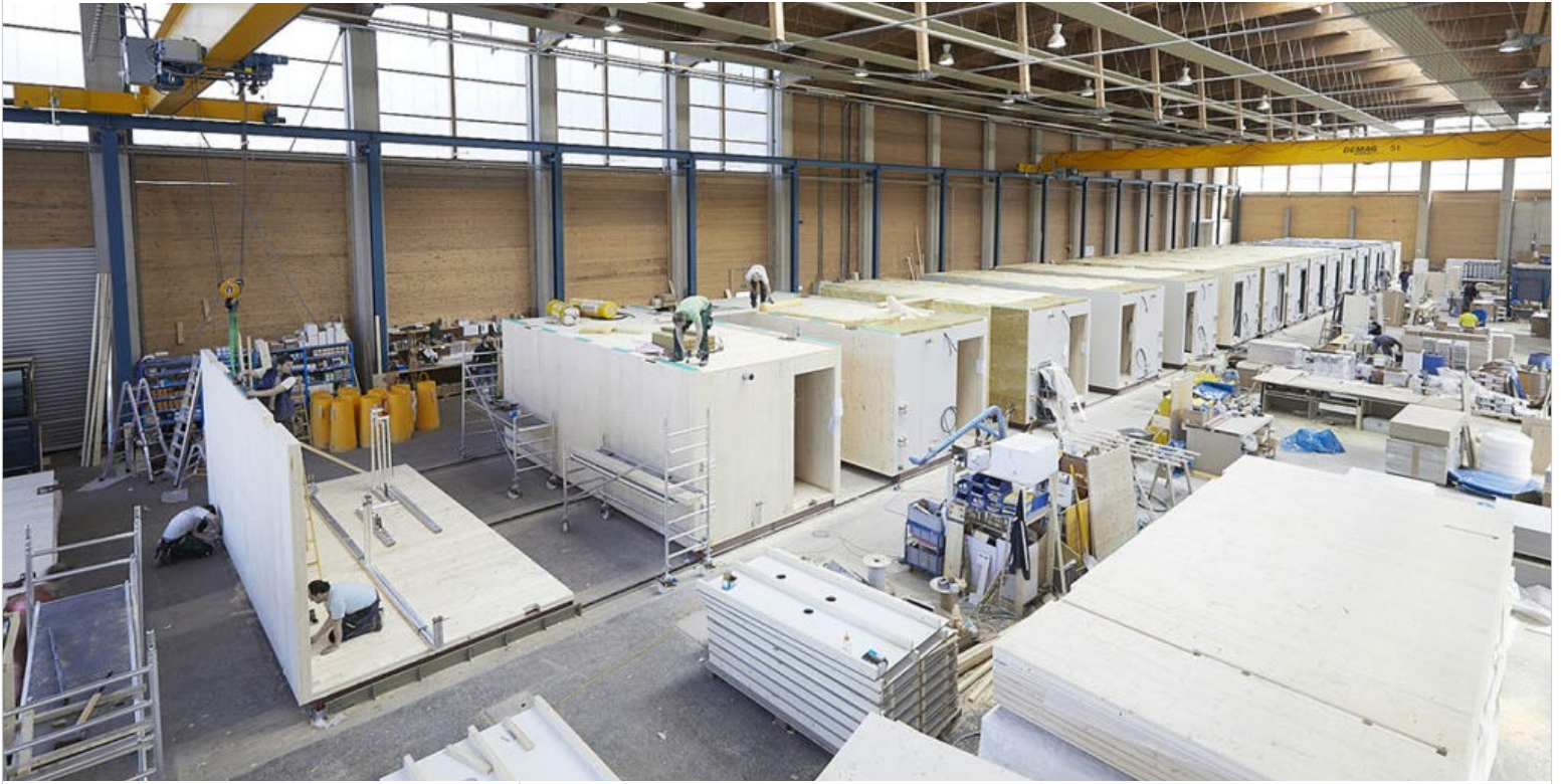
FIG 2: Kaufmann Bausysteme's 3D module production.
